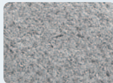
Fig. 47: SEM picture of sandblasted surface of Lava™ Zirconia (Magnification 500 fold).
