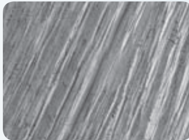
Fig. 35: Lava™ Plus Zirconia ground with a red ring diamond bur (500 fold magnification).
